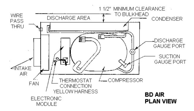
An un-ducted unit in a poorly ventilated small space will heat the air, lowering the cooling capacity and possibly causing damage by overheating the compressor.
